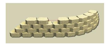
Once the partial unit is in place, glue with a concrete adhesive. Partial units should not be less than 5 inches long and should not be placed directly on top of each other. If the gap is larger than the length of one block, divide the measurement by two and put two partial units in place.
