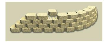
\*To split a block, use a hydraulic splitter or split manually by using a hammer and chisel to score the block on all sides. Pound the chisel on the same line until the block splits. If partial unit sides are not exposed, use a circular cut-off saw with a masonry blade to achieve a tighter fit.
