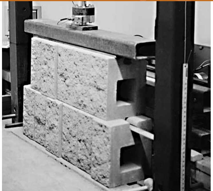
Connection test apparatus with Landmark® modular units.
