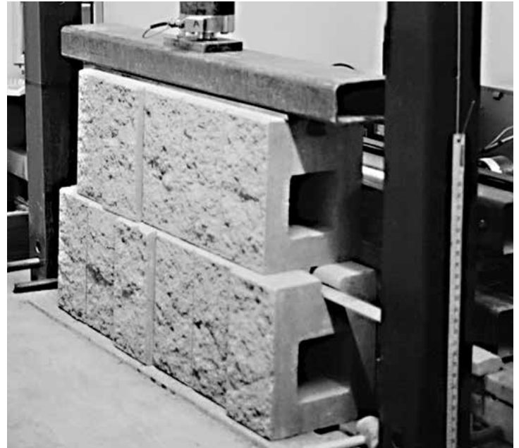
Connection test apparatus with Landmark ® modular units.
