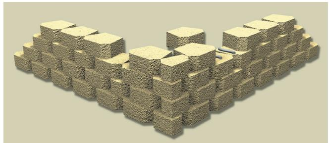
*\*To split a block, use a hydraulic splitter or split manually by using a hammer and chisel to score the block on all sides. Pound the chisel on the same line until the block splits. If partial unit sides are not exposed, use a circular cut-off saw with a masonry blade to achieve a tighter fit.*
