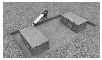
• Set the four units of the second course on top of the first course making sure to line up the corners for a clean edge.
