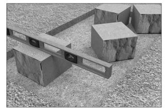
• Place the next end unit back to back with the first unit and level.
