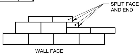
1. ALWAYS START CAPPING WALL FROM THE LOWEST ELEVATION.
