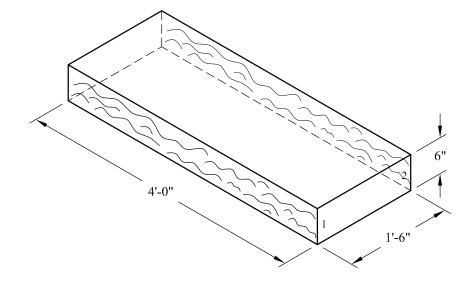
THE TEXTURES ON SIDES 1 AND 2 ARE DESIGNED TO MARRY WITH MINIMAL GAPPING BETWEEN THE UNITS
