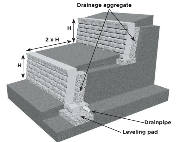
Drainage is vital to maintaining stable, long-lasting terraced walls. Drainpipe must be installed so that the water is directed around or under the lower wall (never place the drain outlet for the upper wall above or behind the lower wall).
