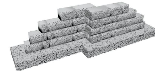
Jogs are used to break up straight lines and add stability to walls. Split units as needed. Use hammer and chisel to round split faces. Glue all courses of jog with a concrete adhesive.
