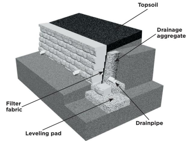
The first category – a gravity wall – is a retaining wall that does not use soil reinforcement. A gravity wall has height limitations specific to each product. An advantage of this type of retaining wall is that it requires a smaller work area behind the wall. A gravity wall relies on the weight and setback of the block to resist the soil forces being exerted on the wall.
