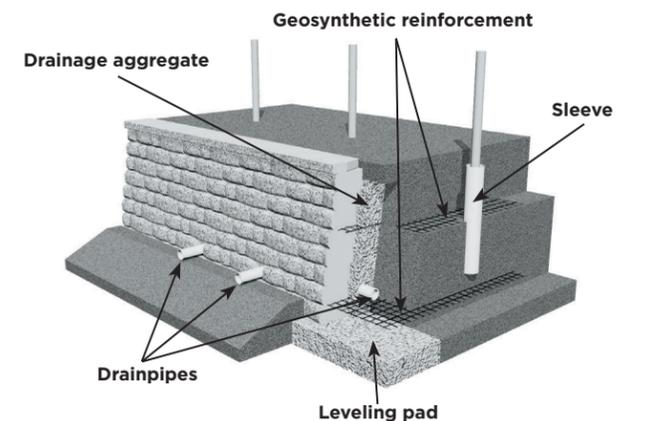
Grout the fence post into the sleeve after the wall is built.
