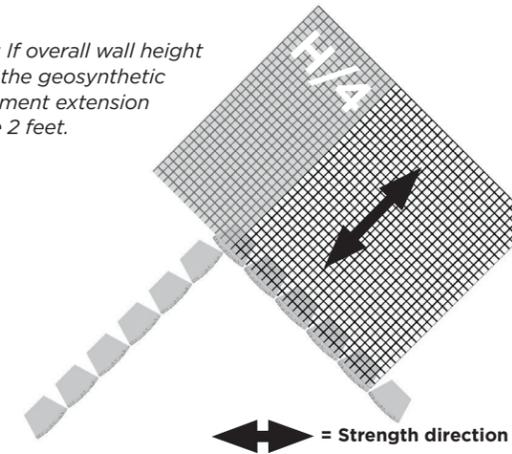
Place the next section of geogrid on the adjoining wall. The geogrid should not overlap and should lie flush with previously placed sections. Once geogrid is in place, the next courses of block can be installed.
