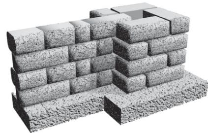
To build columns at the end of a wall, cut one column unit in half for the second, fourth and additional even-numbered courses. Stack column units in a rotating pattern for each course so that the bond is staggered. One column unit half is used every two courses. Glue each course of column units with a concrete adhesive. Integrate wall into column as shown to increase stability.
