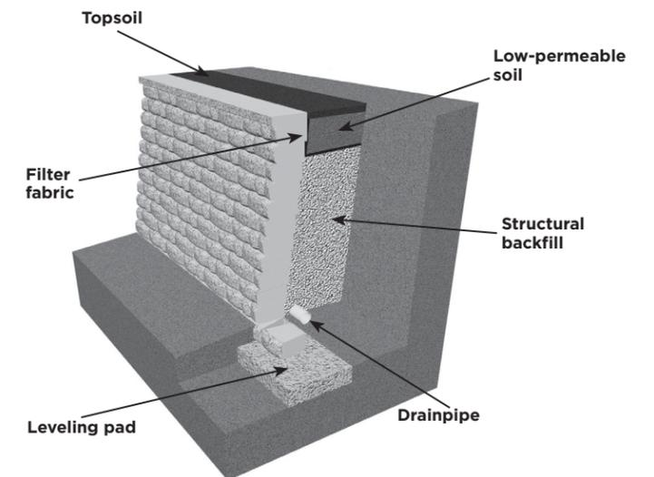
The third category is the Anchorplex™ system, which offers a unique, nonconventional solution to problematic wall construction sites. It is a retaining wall built with Anchor products and structural backfill specified by Anchor Wall Systems, and backed by engineering support tools developed by Anchor.
