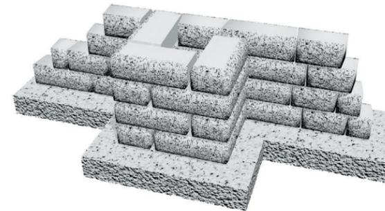
Columns add stability and elegance to a wall. They are located on one side of a wall. To build a column, stack column units in a rotating pattern for each course. Cut wall units as indicated. Glue each course of units in the column with a concrete adhesive.
