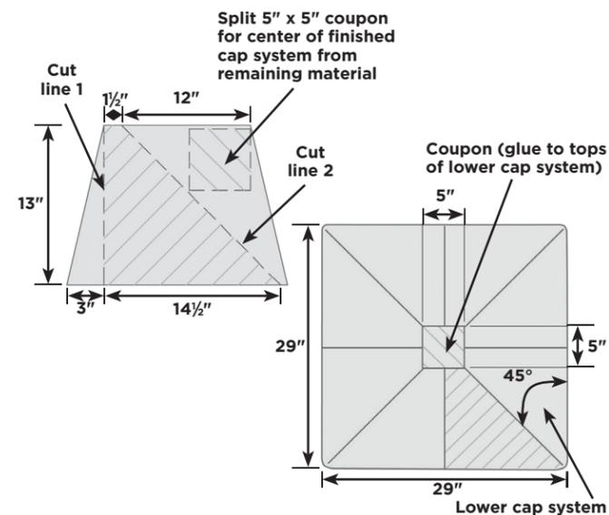
\*\* To split a block, use a hydraulic splitter or split manually by using a hammer and chisel to score the block on all sides. Pound the chisel on the same line until the block splits. If partial unit sides are not exposed, use a circular cut-off saw with a masonry blade to achieve a tighter fit.
