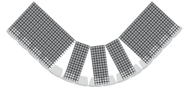
On the second level, fill in the gaps in the first level with strips of geogrid.
