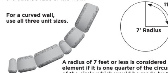
A radius of 7 feet or less is considered a design element if it is one quarter of the circumference of the circle which would be made by that radius (11 feet of a circle with a 7-foot radius).
