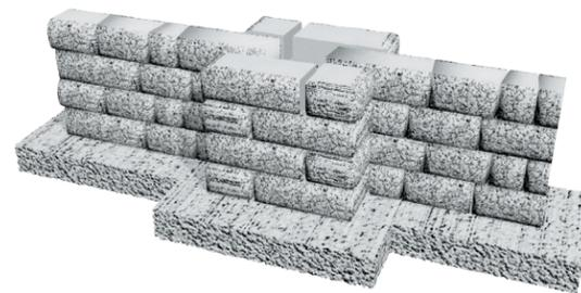
On the first course, use complete column units to start the column and cut the wall units to fit. On the second course, cut two column units in half to fill in the corners. Continue construction by alternating courses. Glue all column courses with a concrete adhesive.
