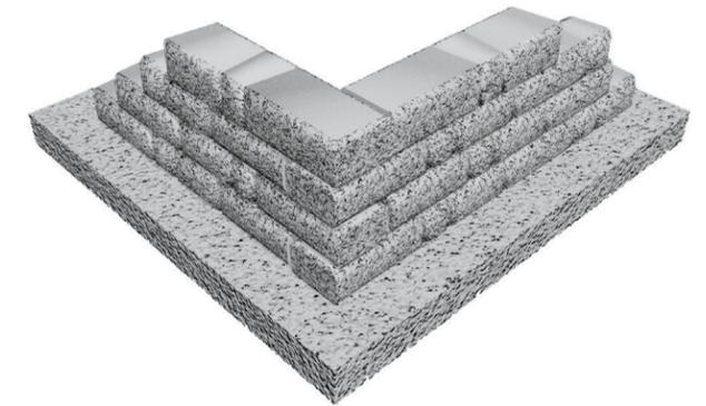
To create a 90° corner in a straight wall, make a third side to a large unit by splitting it to the appropriate dimension. Use only large units to assure connecting units are on bond. Alternate the direction the units face with each course. Round the split ends with a hammer and chisel. Glue all corner courses with a
