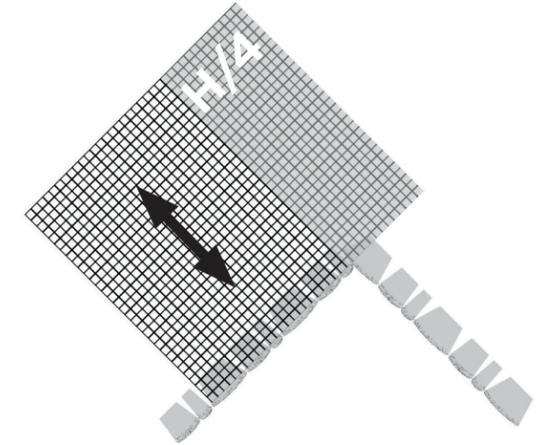
Alternate the geosynthetic reinforcement extension on each course where geogrid is required.
